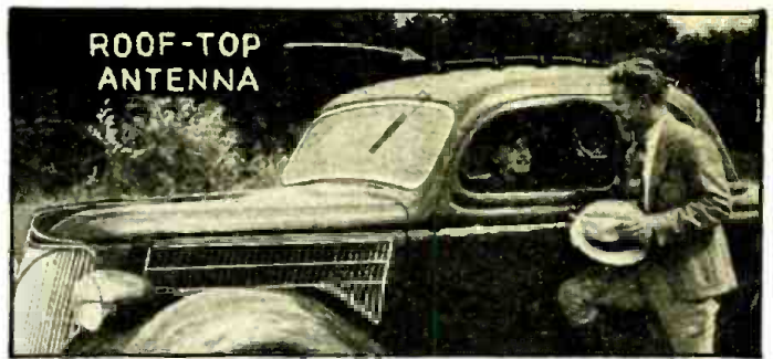
Above and below. New top-of-car antenna improves radio reception. (1043)
